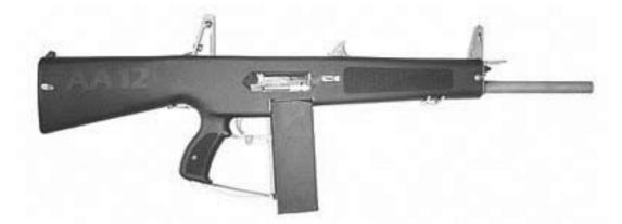
larger than an M4. This wonder weapon requires no tools to maintain it, consists of only eight pieces (including the yard long recoil spring), and feeds from an 8 round box or 20 or 40 round drum. During testing by Blackwater Inc, the gun successfully fed over
